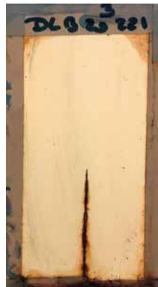
Salt spray resistance after 1000h (Film thickness : 100µm)
