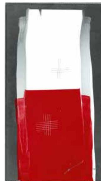
Recoatibility of the primer by a polyurethane topcoat
