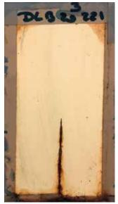
Salt spray resistance after 1000h (Film thickness : 100µm)
