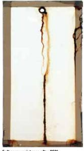
Salt spray resistance after 959h (Film thickness : 85µm)
