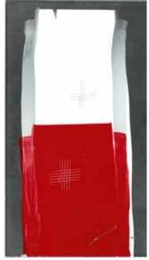
Recoatability of the primer by a polyurethane topcoat
