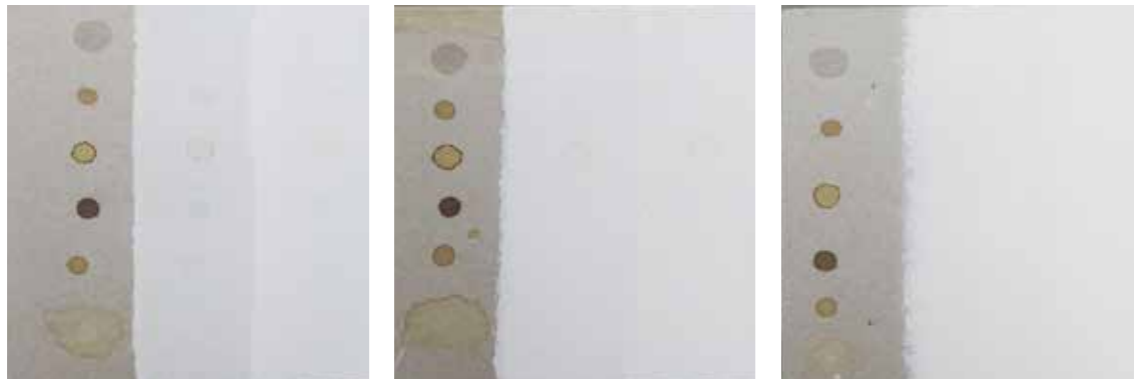
Stain-blocking test of the acrylic classic paint
